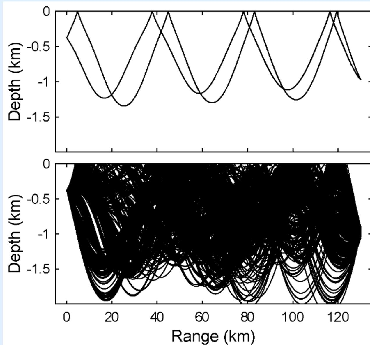
The "small mesoscale" scintillations generate a multitude of eigenrays.
